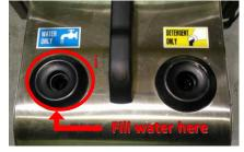
use de-mineralised water, do NOT fill above maximum line indicator (iv) and do NOT fill with any chemicals.
