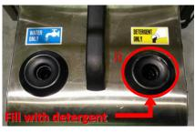
fill with the diluted 101 degreaser solution until it reaches up to the line indicator on the right-side panel (vi). NOTE: We recommend using Steam Australia's 101 degreaser or similar to ensure it does not impact machine operation and/or cause adverse health issues.
