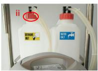
101 degreaser solution up to the top. **NOTE:** We recommend using Steam Australia's 101 degreaser or similar to ensure it does not impact machine operation and/or cause adverse health issues.
