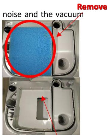
**NOTE:** If the vacuum waste tank lights (b) still flashes after filling the tank up, remove the plastic part with the rectangular hole, then remove the plastic divider underneath. You will see a white float, make sure the white float's surrounding areas and the float itself is clean and can move freely. Re-assemble the waste tank, fill the tank with clean tap water until the vacuum waste tank lights (b) stops flashing then put the blue foam filter and transparent vacuum cover (iv) back on.
