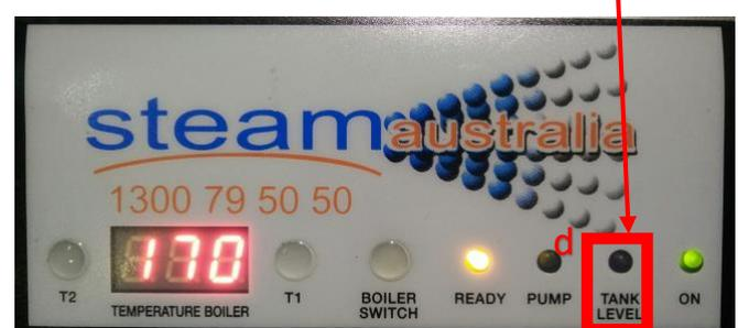
For water tank low level, refer to Step 2 of “Preparing the PEGASO | Steam Operations” (page 1).
