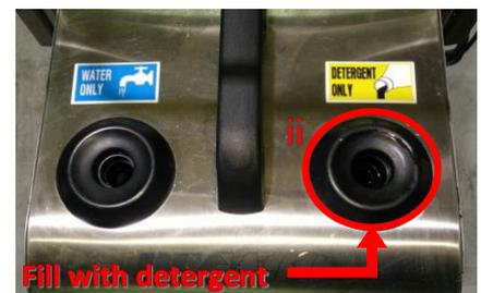
fill with the diluted 101 degreaser solution until it reaches up to the line indicator on the right-side panel (vi). **NOTE:** We recommend using Steam Australia's 101 degreaser or similar to ensure it does not impact machine operation and/or cause adverse health issues.
