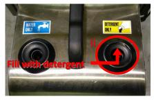
the line indicator on the right-side panel (vi). **NOTE:** We recommend using Steam Australia's 101 degreaser or similar to ensure it does not impact machine operation and/or cause adverse health issues
